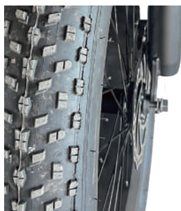
2. Insert wheel into fork.
