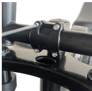
1. Remove the clamp.
