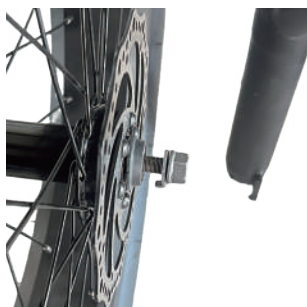
1. Loosen nut fully.
