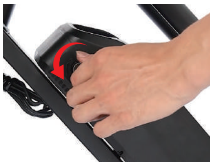
1. Insert key, push in, and turn left.
