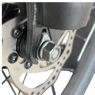
4. Align axle and safety hook.
