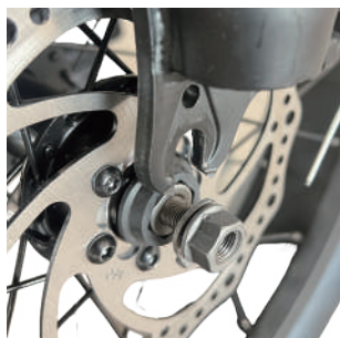
4. Align axle and safety hook.
