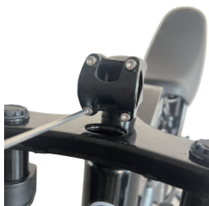
1. Remove the clamp.
