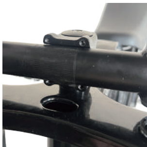
2. Place the handlebar.
