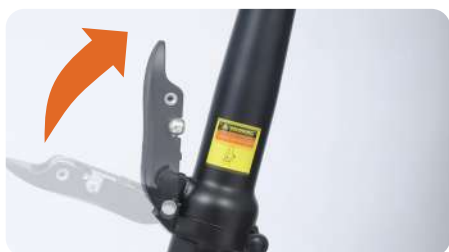
5. Tighten the riser clamp.
