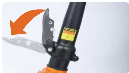
2. Release the riser clamp.
