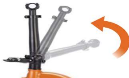
4. Rotate the riser upwards until it fits.
