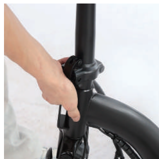
3. Press the locking lever downward.
