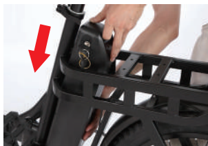
2. Slide the battery down to install.
