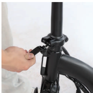
2. Pull the latch upward to the top.
