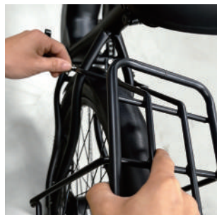
1. Align rack holes and insert bolts.
