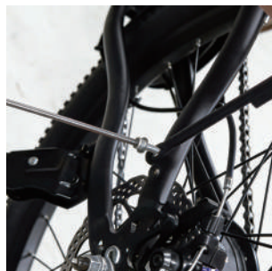
3. Tighten rear bolts on both sides.
