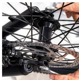
6. Fully tighten nuts.
