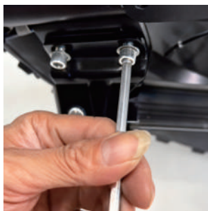
2. Align the kickstand with the frame and install the screws.
