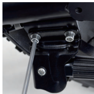
3. Adjust the angle and tighten securely.
