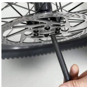
1. Insert axle through hub.
