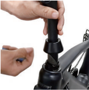
1. Insert stem into head tube.
