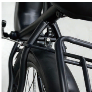
2. Tighten bolts on both sides.
