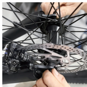
3. Place wheel into fork and align brake.
