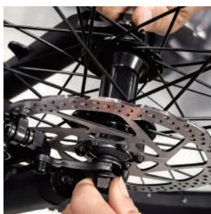
5. Hand-tighten nuts and align hooks.
