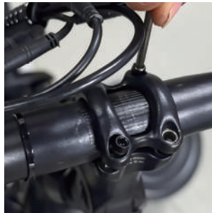
5. Reinstall bolt and cap.
