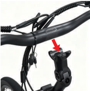
4. Mount handlebar onto slot.
