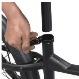
1. Open clamp, insert saddle.
