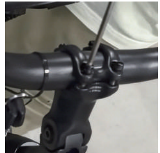
6. Adjust angle and tighten.
