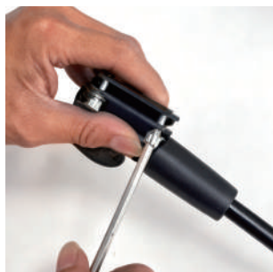
1. Remove two screws from the kickstand.
